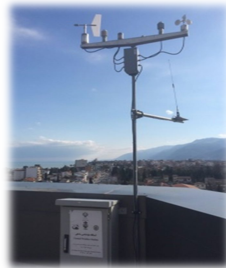
Meteorological and Tide gauge station of Nowshahr port
