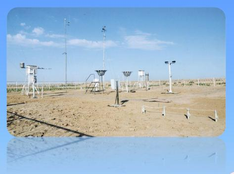
Automatic marine stations installed at existing marine hydrometeorological stations
